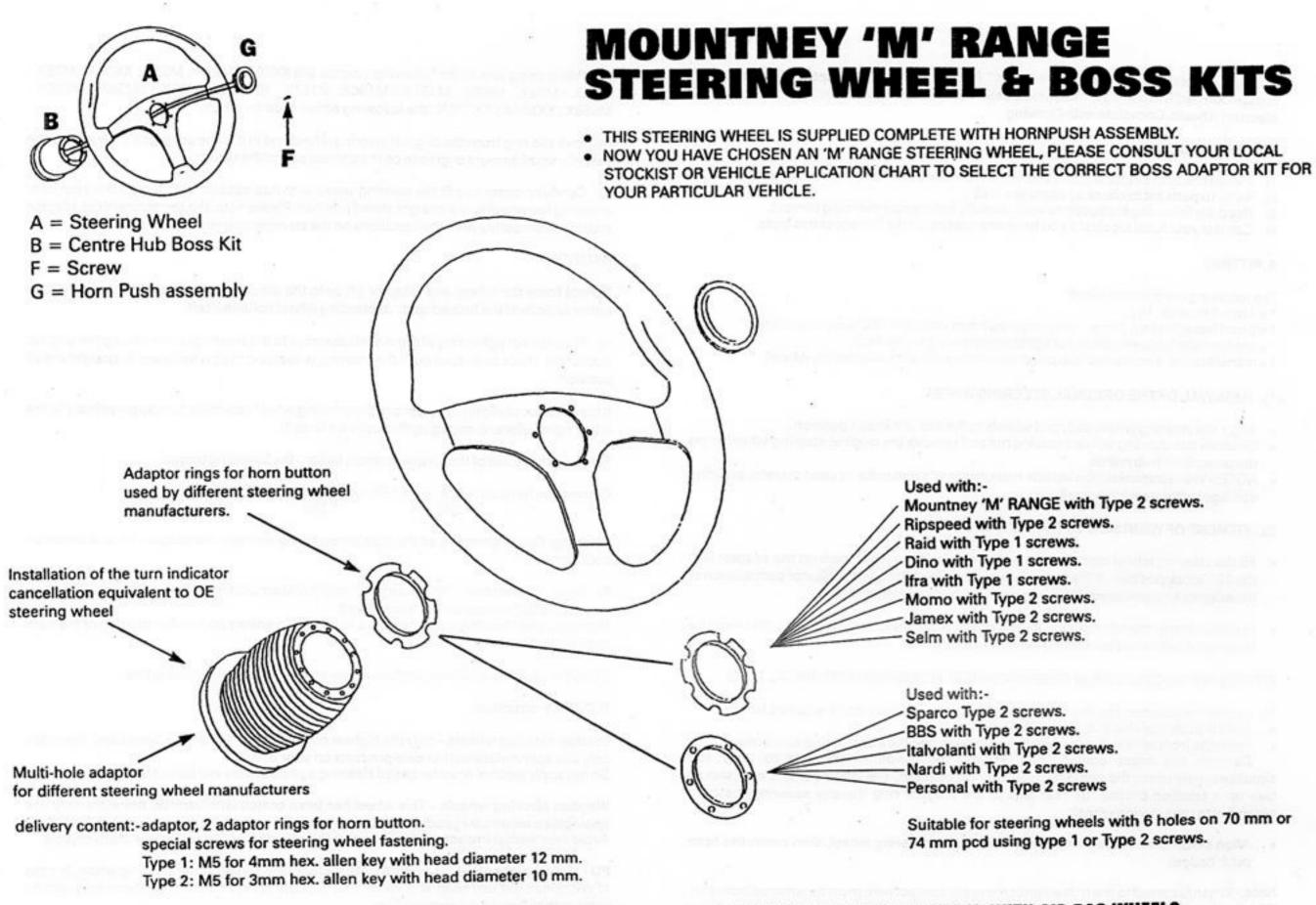
Fitting instructions for the "M" & " KK" Range Multi-hole Adaptor Kit, used with Ripspeed/Raid/Dino/lfra/Momo/Jamex/Selm/Sparco/BBS/ Italvolanti /Nardi/ Personal/ steering wheels. Complete with Drawing.
