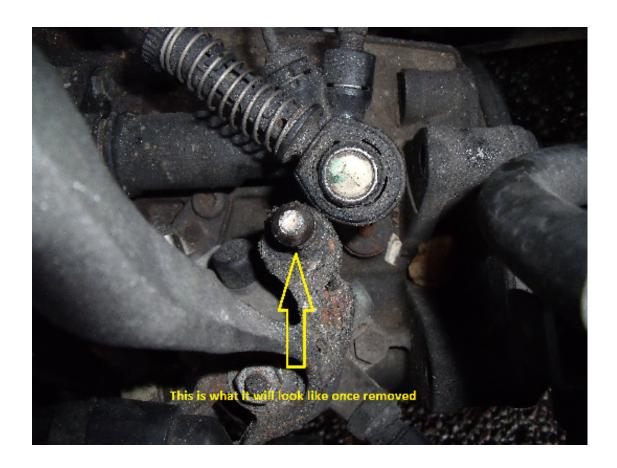
Next remove the circular clip on the side to side shifter mechanism as pictured below. and pull this back a few centre meters to give you enough room to remove the shifter
