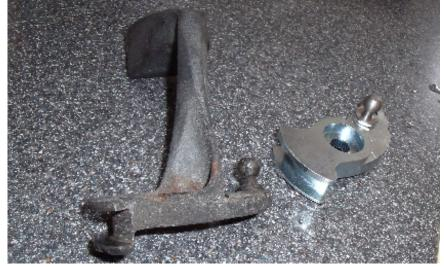
Once both OEM linkage components are removed, you will need to assemble the Forge replacement linkage components that you intend to install.
