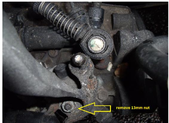
Once the 13mm nut is removed, slide the front-to-back linkage up off of the splined selector shaft. This will take some force and it is recommended to rock the linkage from side to side very slightly in order to loosen it, but please do not use a hammer or anything else to pound or tap the shaft out of the bottom of the linkage as this may lead to damage to various components. Though it will take some effort, the linkage will certainly come loose within a short time.
