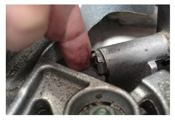
Next undo the 13mm nut that is securing the shifter to the gear box as pictured below
